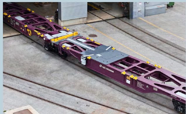
Railrelease's new "Power Wagon", featuring an underfloor configuration
